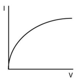
We can see the graph is not straight but is **curved**. As a potential difference is applied across a lamp, a current begins to flow in the lamp causing it to light. However, this current flow means some heat energy is dissipated in the filament. This causes the filament to heat up and then the **resistance increases**.
