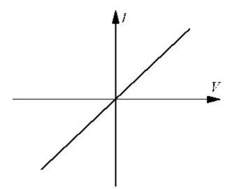
This graph shows that the current is directly proportional to potential difference and so the resistance is constant as current increases. Therefore, a metal wire at a constant temperature is an **ohmic conductor**.
